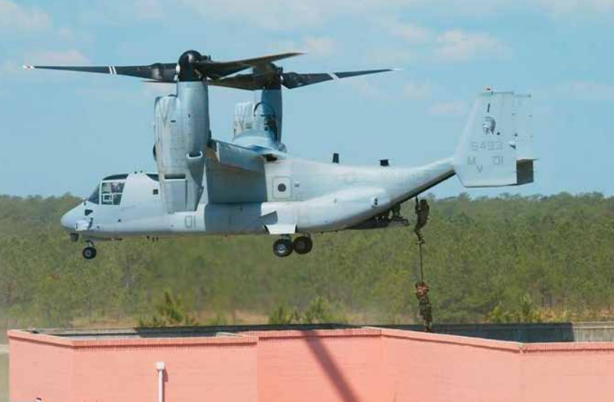
Fast rope system at the rear cabin
