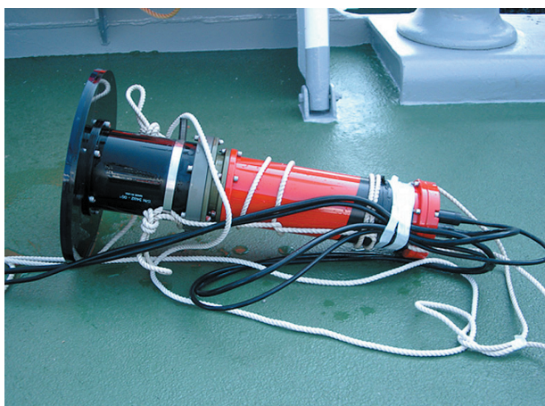
Fig. 3 Current acoustic transducer employed on the on-board unit.
