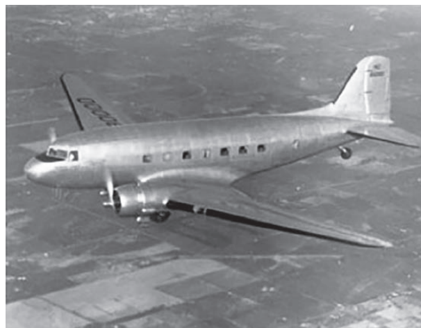
Fig. 2 DC-3, the first aircraft to use Alcoa's Alclad 24S-T3 on the fuselage 20) .
