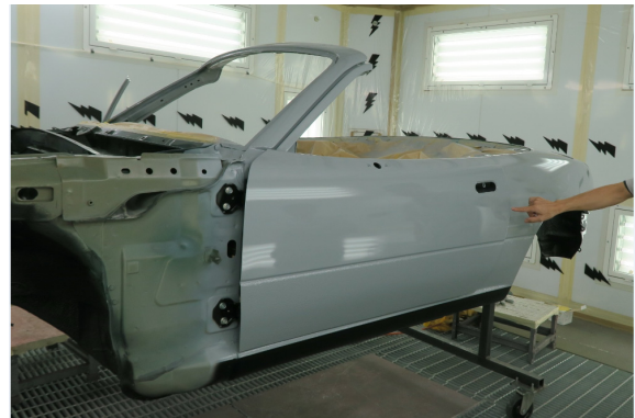
Fig. 6 Before Top Coating
