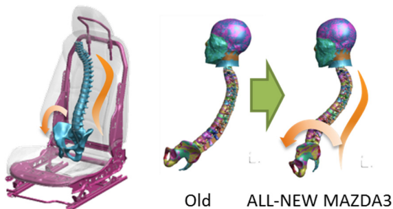
Fig. 7 New Seat Structure & S-Shaped Alignment of Spine
