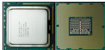
Intel Core i7 microprocessor (around 781 million transistors)
