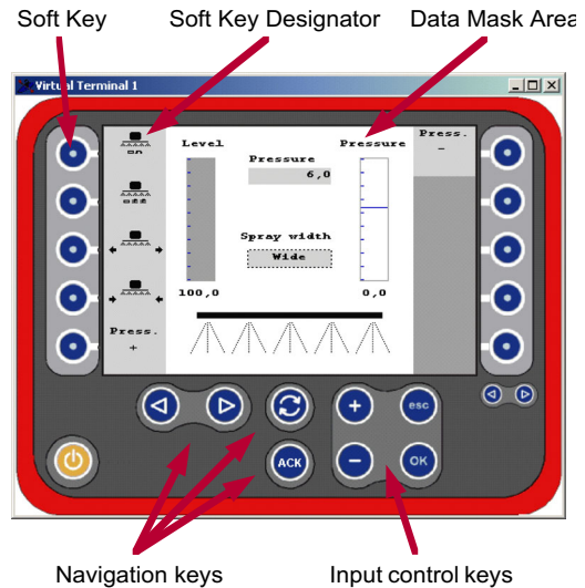
Figure 2 – Simulated VT with CANoe
