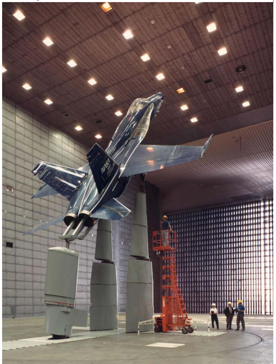
▲ An F/A-18 fighter aircraft is tested for high angle-of-attack aerodynamics in the 80-by-120-foot wind tunnel at NASA's Ames Research Center in California. NASA
