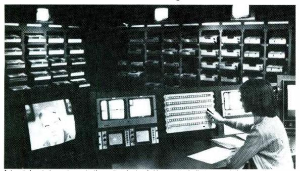
Automated control console constantly monitors banks of videocassette duplicators seen in background at the new Teletronics Video Services facility in Des Plaines, III. Electronic routing switcher shifts signals through plant.
