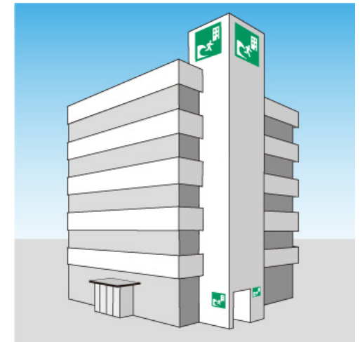
Example of the sign installed at 1 st -floor and top of the building f) Installation example of tsunami evacuation building sign
