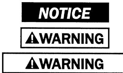
Figure B1 Examples of Correct Safety Alert Symbol and Sign Word Placement
