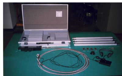
Type II life-saving system (Component: Equipment to detect presence of persons within damaged structures)
