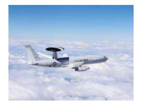
3 fills the needs of both command and control (C2) functions for tactical and air defense forces. The E-3 offers superior surveillance capabilities. Equipped with a "look-down" radar. The AWACS can separate airborne targets from ground and sea clutter returns. It also can detect and track both air and sea targets simultaneously. AWACS has earned the reputation as an international keeper of the peace.
