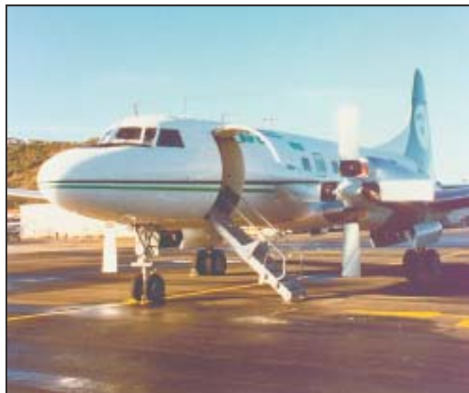
Below: Civil operators of the T56 in New Zealand include Convair 580 operators. The airframe was originally powered with Pratt and Whitney R2800 engines. An extensive STC programme saw a number of turbine engines tried, the most common being the Allison T56.
