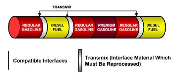
There is always a certain amount of intermixing between the first product and the second at the "interface," the point where they meet. If the products are similar, such as two grades of gasoline, the resulting mixture is added to the lower value product. If the products are dissimilar, such as diesel and gasoline, the "transmix," the hybrid product created by intermixing at the interface, must be channeled to separate storage and reprocessed.
