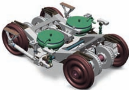
Trailer bogie: Only 2,100mm wheelbase and the very low weight of the new bogie design lead to significant improvements in energy consumption, track-friendliness and wheel wear.
