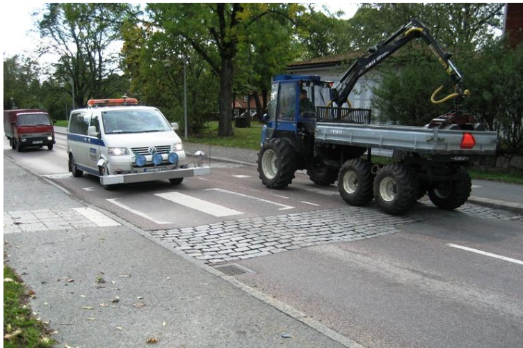
Figure 1. Profiling a flat top bump with cobble stone with the Profilogaph.
