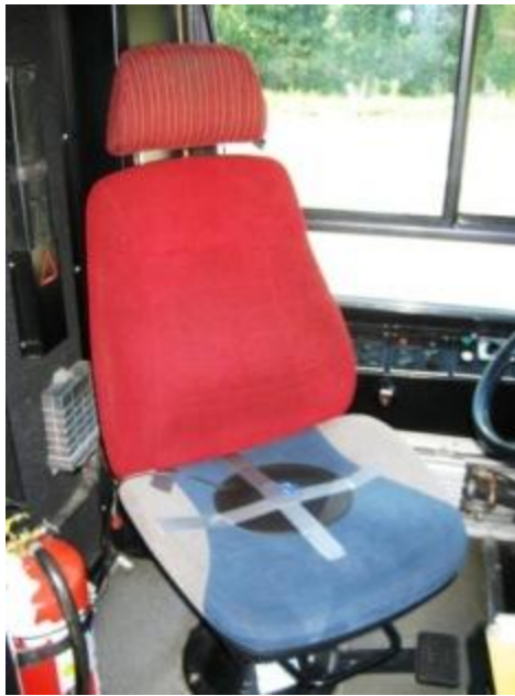
Figure 3. Triaxial seat pad mounted on the bus driver's seat.
