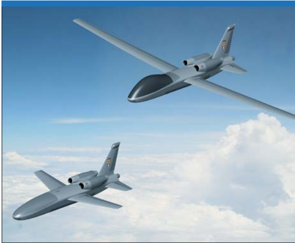
The Eads Modular Advanced UAV will consist of a single 10.3-metre backbone fuselage cum engine and tail unit to which 25.25-metre span wings can be fitted for 46,000-ft altitude missions. Endurance would be around 17 hours. The 'canopy bay' would receive a Ku-band satellite aerial. The shorter set of wings (about nine meters) will provide high-speed low altitude (1000 ft) dash missions. (Eads)
