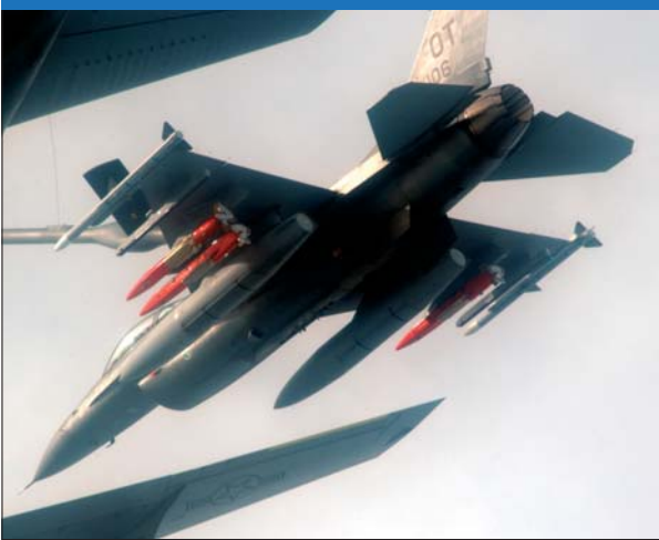
The swing-wing Raytheon AGM-160B Mald (Miniature Air-Launched Decoy) has a range of 925 km and been cleared for use on the Lockheed Martin F-16 (shown here) and the Boeing B-52. (Raytheon)
