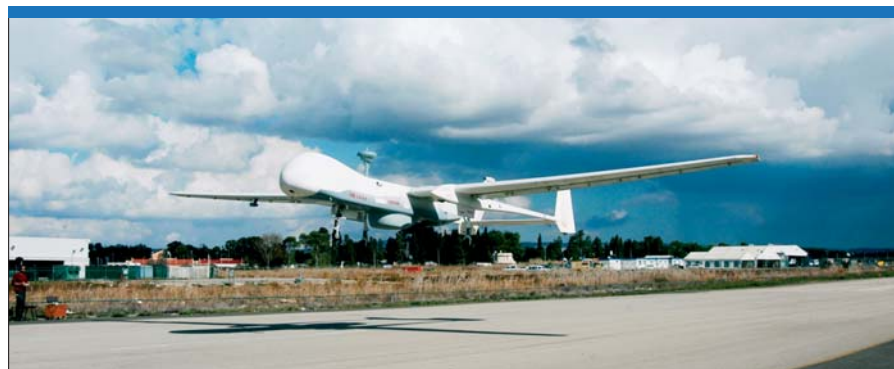
This recent photograph of an IAI Heron I shows it camouflaged light blue on the undersurfaces and painted white on top, presumably to reduce the heating produced by solar radiation. (IAI)
