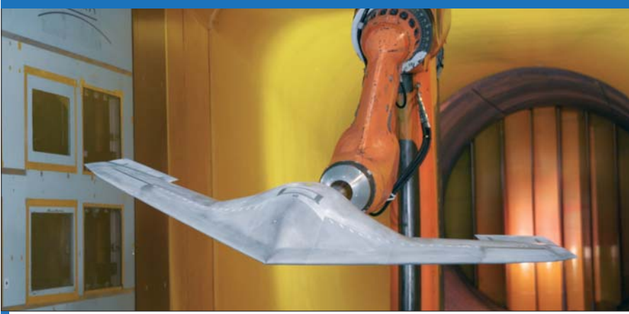
A wind tunnel test model of the Neuron is here seen being put through its paces at Onera's facilities in France. As for its American counterpart, low radar signature is a mission prerequisite. (Dassault)
