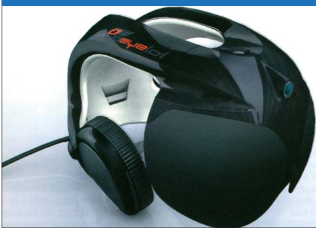
Innosuisse has developed a pilot helmet called Peyelot to help the operator to virtually slide into the skin of a drone. Linked to the ground control system, the helmet is equipped with a display and the onboard camera is slaved to the helmet's movements. (Innosuisse)
