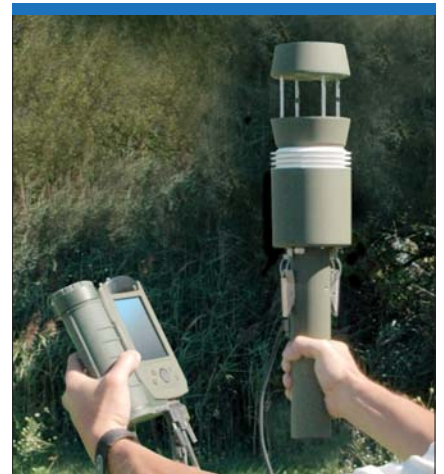
The Tacmet II, from Climatronics, is seen here used in conjunction with a PDA. The solid-state Tacmet II can also be used on a tripod to provide a nearby mobile control station for wind, temperature, relative humidity and barometric pressure data. (Climatronics)
