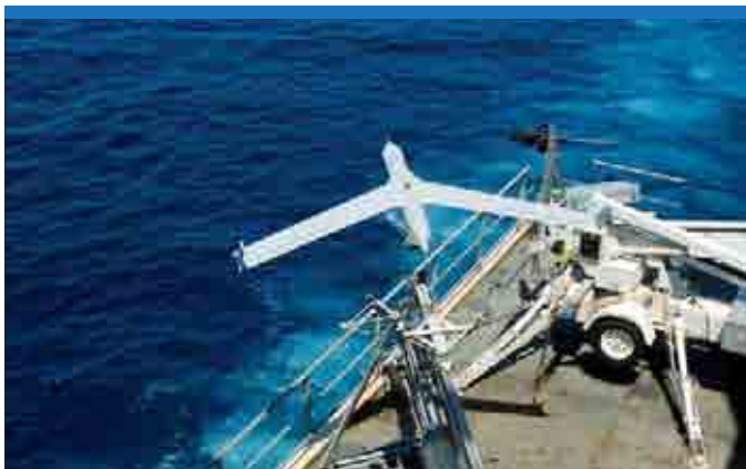
One of the most significant developments in the 20-kg category has been the Insitu Insight, which provided the basis for the 18-kg Boeing/Insitu Scaneagle and its launch and recovery system. (Insitu)
