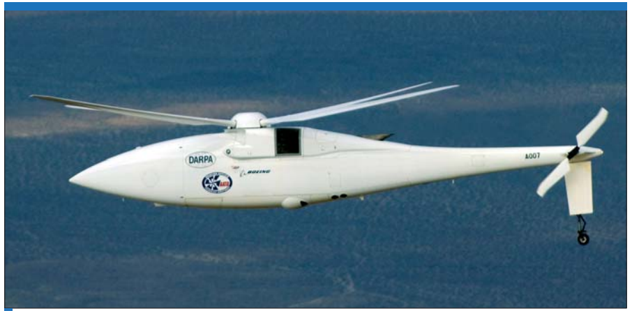
The Boeing A160T Hummingbird is a turbine-engined development of the piston-engined A160 designed by Frontier Systems. It is hoped to produce a breakthrough in rotorcraft speed, ceiling and endurance. (Boeing)
