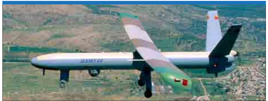
The parasol-wing, fixed-gear Hermes 450 entered service with the Israel Defense Force in 2000. It has also been purchased by Botswana and Singapore, and has been leased by the British Army. (Elbit)
