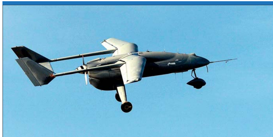
The Selex Galileo Falco was cleared following 18 flight tests made by the end user (believed to be Pakistan) during which it carried out a surveillance mission at maximum payload which lasted 9 hours and 15 minutes, demonstrating, by using an auxiliary fuel tank, maximum endurance could exceed the 14 hour mark earlier anticipated. (Selex Galileo)
