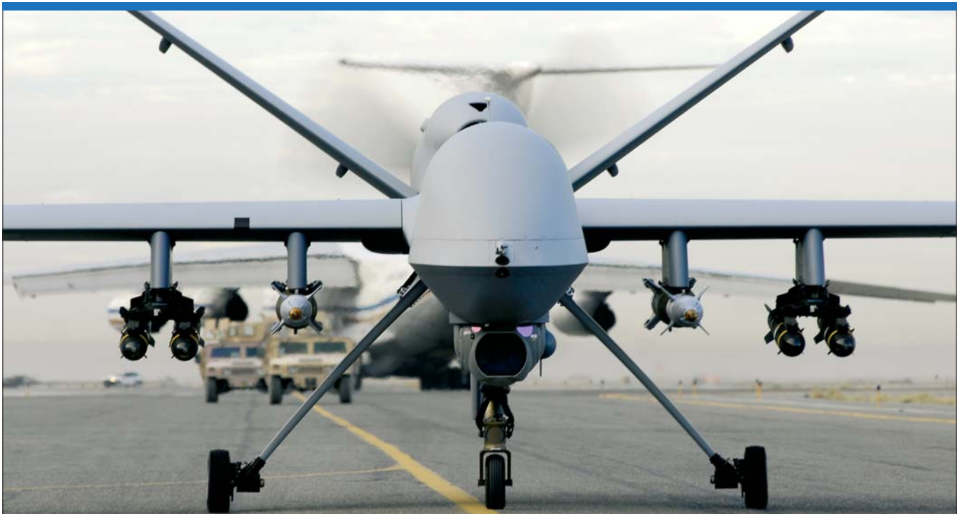
Deliveries of the General Atomics MQ-9 Reaper to the US Air Force began in March 2007. A Reaper is shown here in Afghanistan armed with Hellfire missiles and GBU-12 Paveway II laser-guided bombs. (General Atomics)
