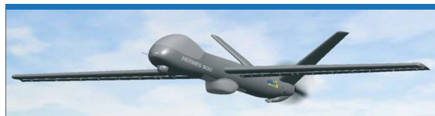
The 970-kg Elbit Systems Hermes 900 is a larger, retractable-gear, mid-wing derivative of the 550-kg Hermes 450. Unveiled at the Paris Air Show in 2007 it was to fly in early 2008. (Elbit)
