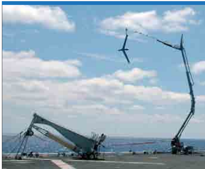
On the USS Saipan (LHA-2) amphibious assault ship, this Boeing/Insitu Scaneagle, launched from the catapult on the left, has just been recovered by engaging a cable suspended from the Skyhook rig. (US Navy)
