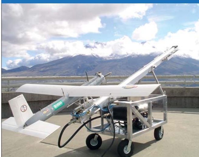
The 9.1-kg Advanced Composites Research Silver Fox is to be purchased for the US Navy, US Marine Corps, US Army and Socom. This example was being used by the US Geological Survey. (Advanced Composites Research)
