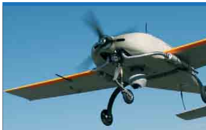
Seen here under the Raytheon experimental Cobra, the KJ600 has also been tested in the Swift Killer Bee, the Arcturus T-16 and the Snow Goose. (Optical Alchemy)
