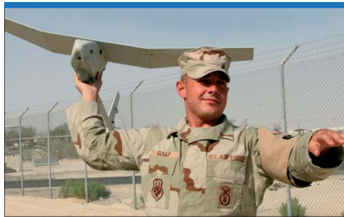
The AV RQ-11B Raven-B is the current leader in the hand-launched drone category, with well over 5000 already delivered and production heading for more than twice that number. (US Air Force)
