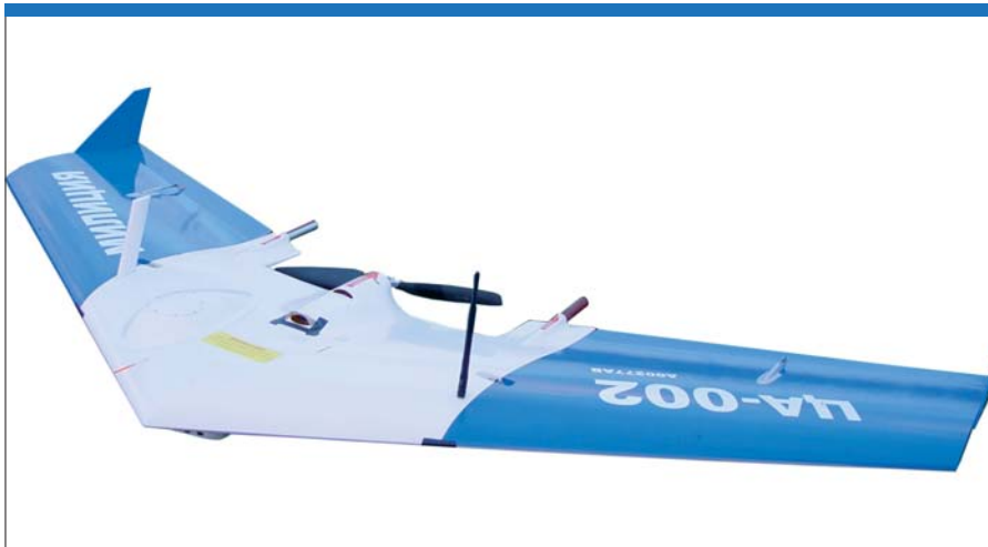
Russia's principal hand-launch drones appear to belong to the A-Level Aerosystems Zala 421 family. The 2.1-kg Zala 421-08 is used by the Interior Ministry, and this 421-04 weighs up to 7.9 kg. (A-Level Aerosystems)
