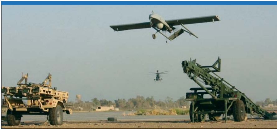
The 170-kg AAI RQ-7B Shadow 200 has served with the US Army since 2002 and has also been adopted by the US Marine Corps to replace the RQ-2 Pointer. It is launched from a ten-metre rail. (AAI)
