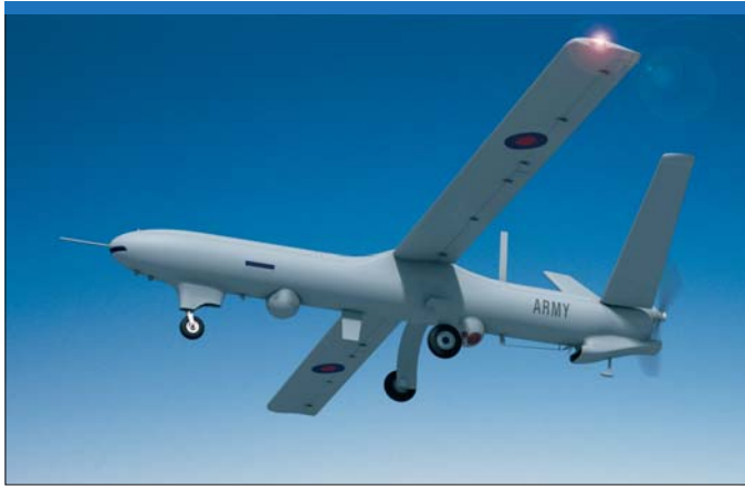
This impression of the British Army's Thales Watchkeeper shows some differences from the Elbit Hermes 450: the shoulder-mounted wing, retractable nose gear and twin sensor turrets. (Thales UK)
