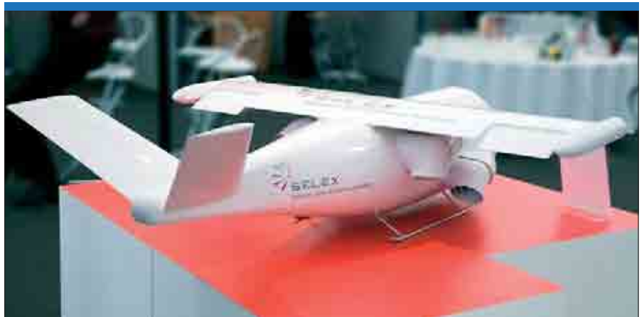
Unlike tail-sitter ducted fan projects, the Selex Galileo Damsselfly is a flat-riser using four rotating nozzles (as in the Rolls-Royce Pegasus), with the aft nozzles raised to avoid interaction of the jets. (Selex)
