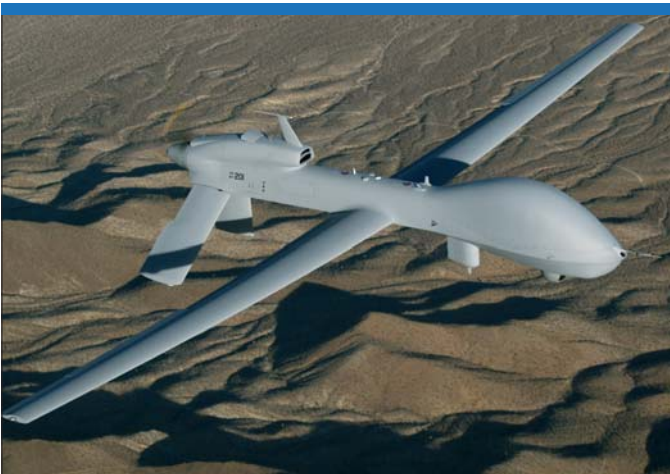
The MQ-1C Sky Warrior differs from the Predator in having a Thielert diesel HFE (heavy fuel engine) and atol (automatic take-off and landing) facility, to avoid the need for a qualified pilot. (General Atomics)
