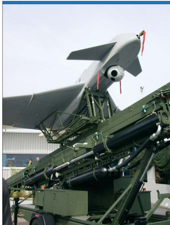
A successful programme, the Sagem Sperwer has seen extensive deployment in former Yugoslavia and now in Afghanistan. The French manufacturer is now looking into the development of a Mk II with extender range and a sharper electro-optical sensor. (Armada/EHB)
