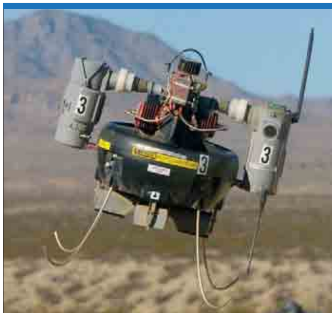
The shape of things to come? Successful evaluation in Iraq of the Honeywell G-Mav (gasoline-powered micro air vehicle) has led to a US Navy order for 186 production RQ-16A systems. (US Navy)
