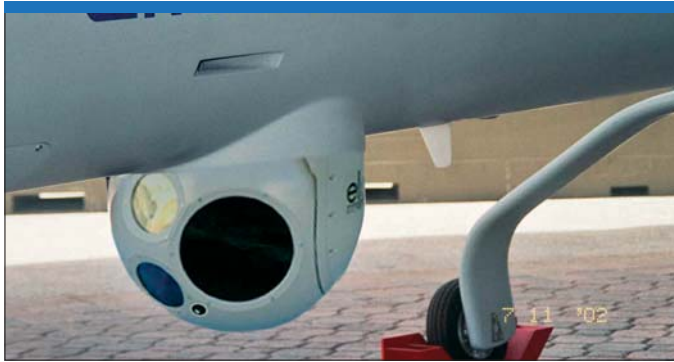
The Compass IV is Elbit's top-of-the-range gimbal sensor for drone applications. It weighs 38 kilos and is here seen under a Hermes 450 from the same company. (Elbit)
