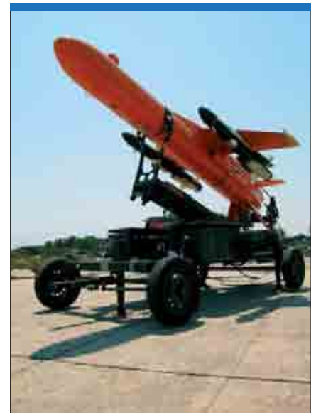
The use of a drone to launch mini-targets is represented by this 330-kg Meteor Mirach 100/5, carrying two 20-kg Selex Galileo Locustas, as used to test German Air Force Patriot missiles. (Selex Galileo)
