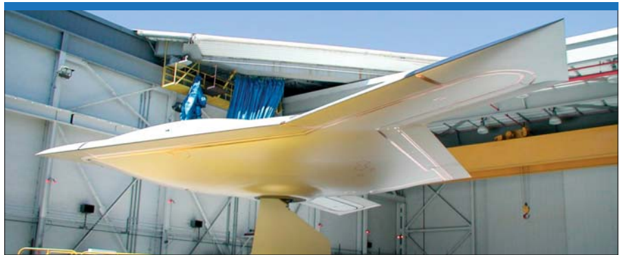
Paving the way for the US Navy's next strike aircraft, Northrop Grumman's unmanned, subsonic X-47B demonstrator will rely heavily on its low radar signature, shown here under test. (Northrop Grumman)
