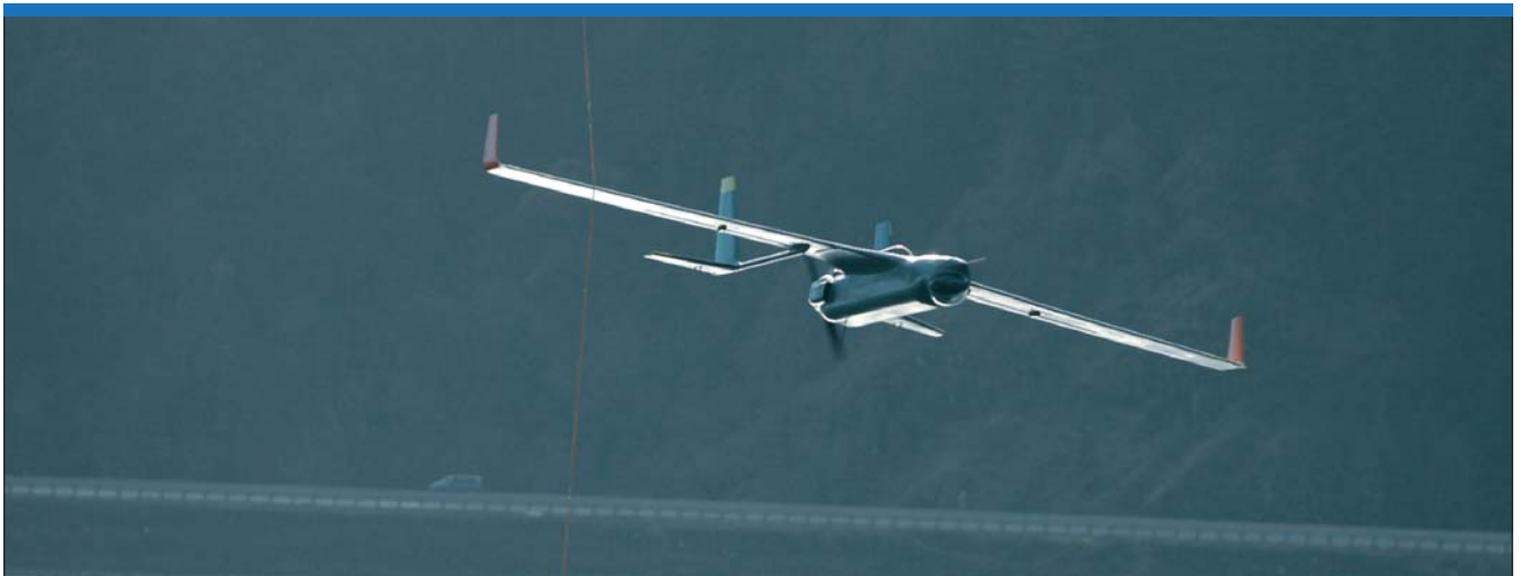
Building on Scaneagle experience, Insitu sees the way ahead as a far heavier (59 kg) conventional twin-boom configuration. This Integrator prototype flew in August 2006 and a near-production aircraft appeared a year later. (Insitu)
