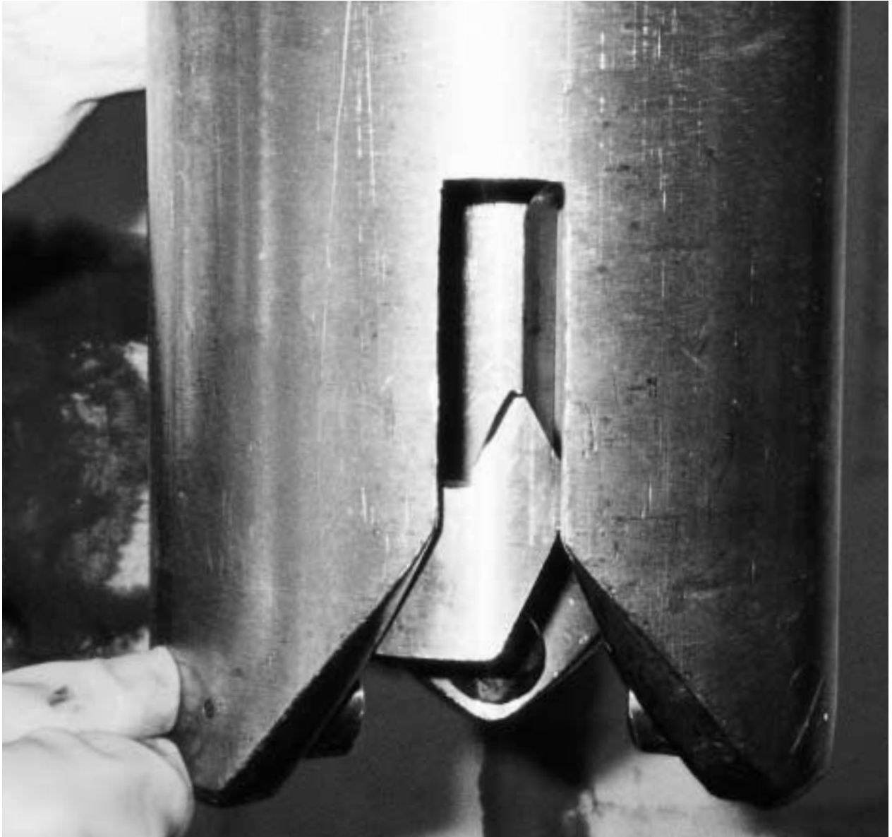
Figure 4: Jaws of the basket grab in partially closed position
