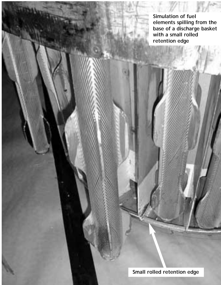
Figure 7: Fuel elements inside discharge basket
