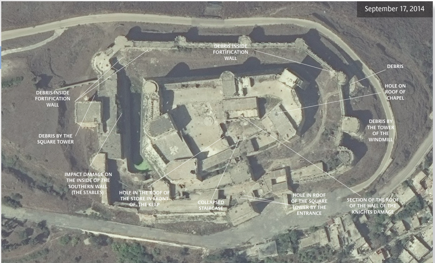
FIGURE 31. Overview of Crac des Chevaliers and locations where damage has occurred and is visible.
