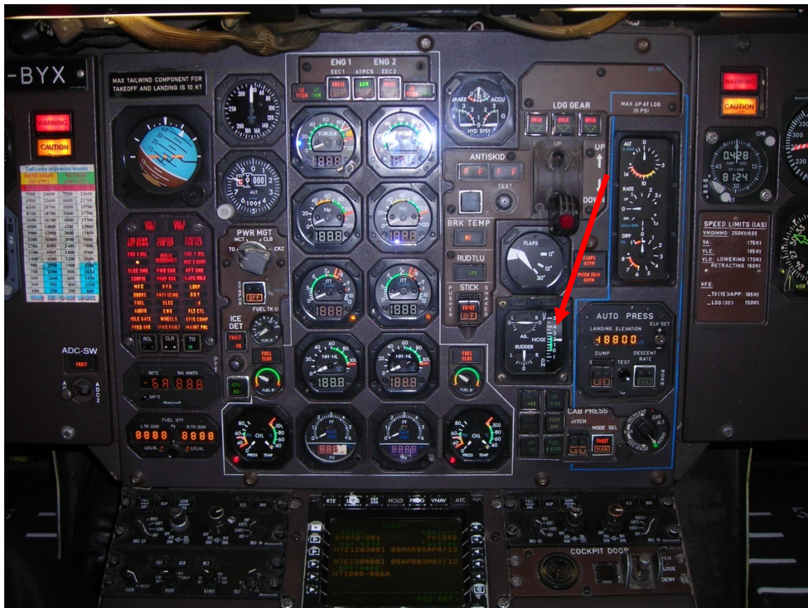
Figure 59. The instrument panel with the indication of the elevator trim position
