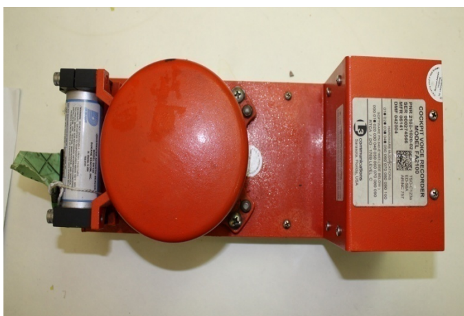
Figure 5 Cockpit Voice Recorder (CVR) FA2100 SN000274566
