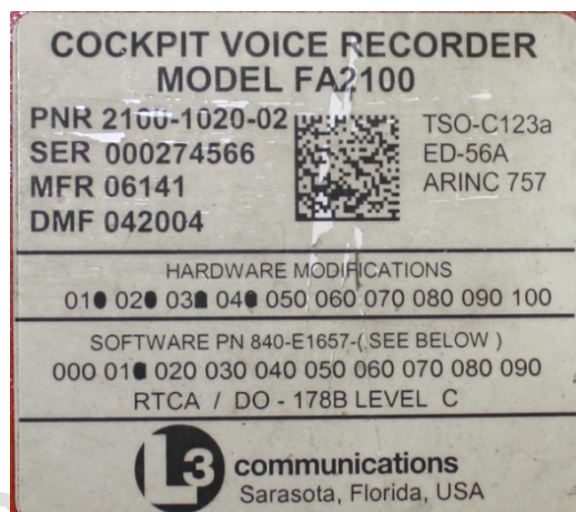
Figure 6 CVR identification label
