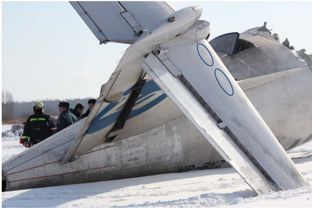
Figure 1. Horizontal stabilizer right side with traces of snow and ice deposits
