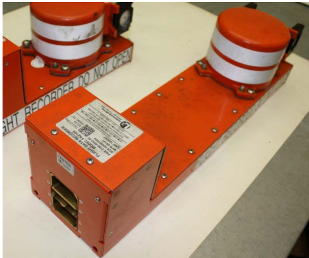
Figure 7 Flight Data Recorder (FDR) FA2100 SN000501604
