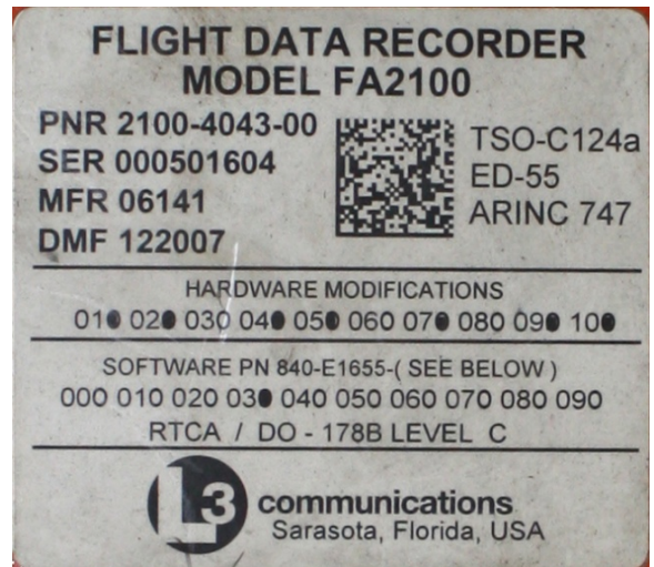
Figure 8 FDR identification label
