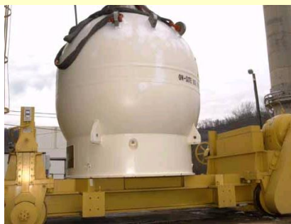
25-ton Q-ball transporting irradiated Am/Cm seed material
