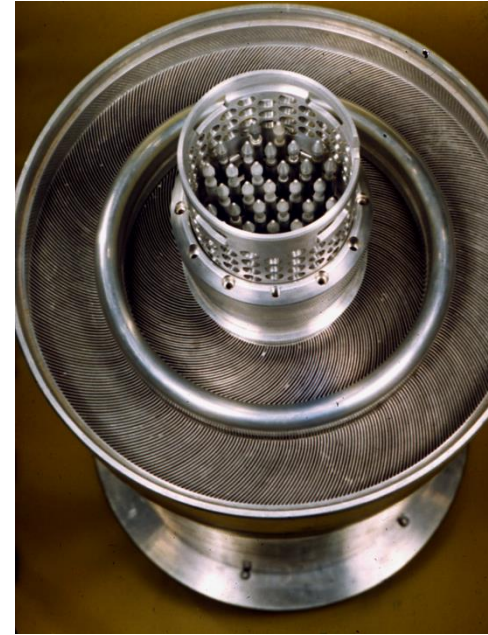
Target positions in the flux trap of HFIR fuel assembly
