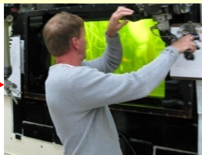
Chemical separation in hot cell REDC, ORNL, Oak Ridge
