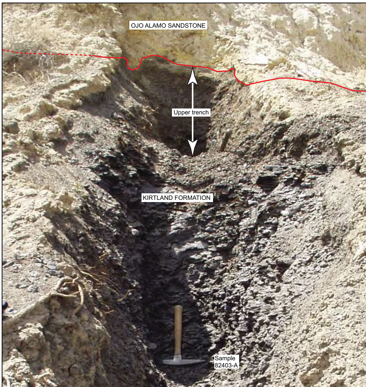
Figure 62. Photograph of trench cut through base of Ojo Alamo Sandstone and uppermost Kirtland Formation at Barrel Spring locality. Figure 61 shows location of trench. Sample locality 82403-A is about 4 m below base of Ojo Alamo Sandstone at about same stratigraphic level as coaly bed that pinches out east of here (Figure 61). Contact between Ojo Alamo Sandstone and Kirtland Formation shown by red line (solid where clearly visible, dotted where covered). Geologic pick 0.33 m long.
