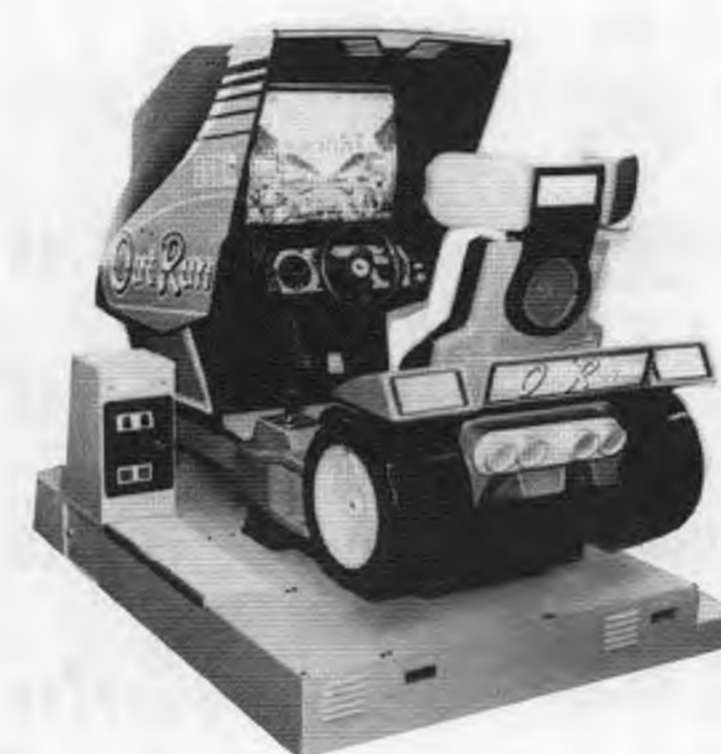
Photo above: Sega's "Out Run" (deluxe type) inclines left and rightward according to the player's handle control.
