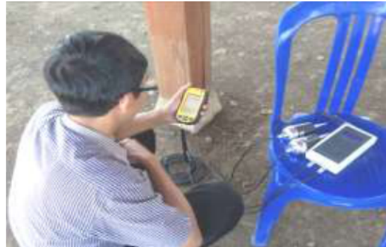
Figure 8. The process of reading the test data in the Sylvatest TRIO instrument (Source: authors)
