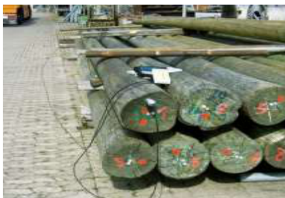
Figure 4. New-wooden-poles quality evaluation using non-destructive testing (Benoit and Sandoz, 2011)
