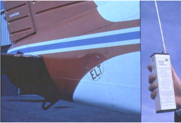
An automatic ELT is often installed in the aircraft tail section, which is assumed to better survive a crash.
