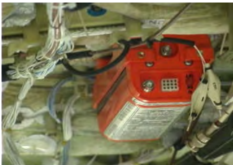
406 MHz Aircraft ELTs Installations
