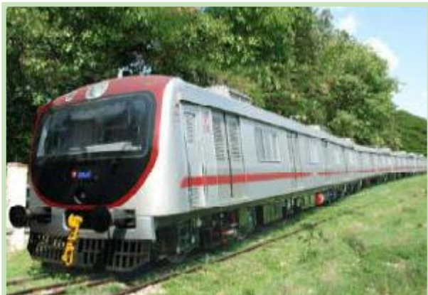
Unpainted metro-car in Austenitic Stainless Steel (Photo: Indian Stainless Steel Development Association)
