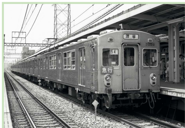
Japan's first all-stainless steel railcar (Tokyu's 7000-series) (Photo: Tokyu Car Corporation)
