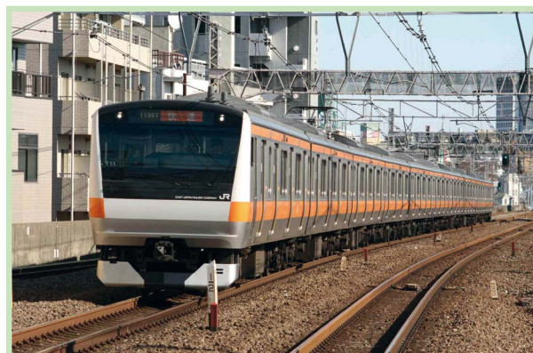
Recent stainless steel commuter train (JR East Japan's E233) (Photo: Tokyu Car Corporation)
