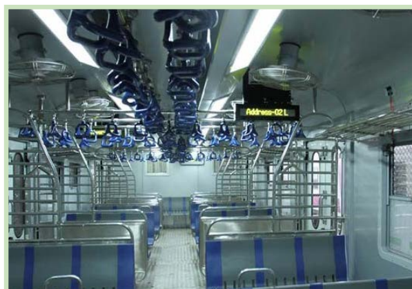
Intercity EMU Trains : All interiors made in stainless steel (Photo: Indian Stainless Steel Development Association)
