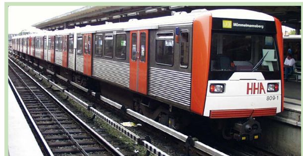
Positive long-term experience with the DT-3 ensured Hamburger Hochbahn opted for stainless steel in its next generation of trains (Photo: Hamburger Hochbahn AG)
