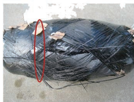
Validation through burst test
