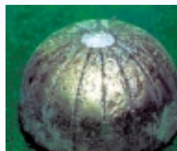
Half sphere of as-cast \delta -plutonium alloy
