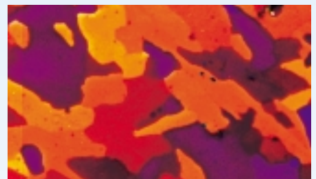
Polycrystalline \delta -phase plutonium alloy
