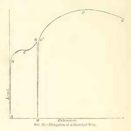
The part of the increment of elongation which disappears on the removal of the stretching weight, between the elastic limit and the yieldpoint, is proportional to the stretching weight, and the ratio of this movement to the stretching weight per unit area is, according to the experiments of Professor Kennedy, the same as that within the limits of perfect elasticity (see Todhunter and Pearson's History of Elasticity, p. 889).
