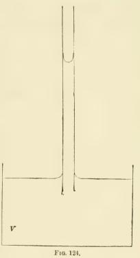
to which the liquid rises in the tube. To measure r, the radius of the tube at the level of the meniscus, cut the capillary tube carefully across at this point and then measure the internal radius by a good microscope with a micrometer scale in the eyepiece. If the section, when observed in the microscope, is found to be far from circular, the experiment should be
