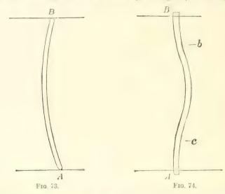
the ends must be parallel to the line of action of the force, and there must be two points of inflection at, b and c; hence the distance between the ends is twice the distance between two points of inflection, so that
