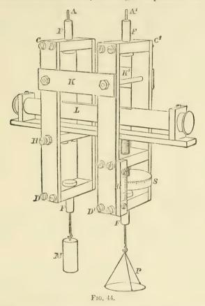
wire A' is stretched, and the bubble moves towards H; bring the bubble back to zero by turning the screw; the distance through which the screw is moved is equal to the extension of the wire.
