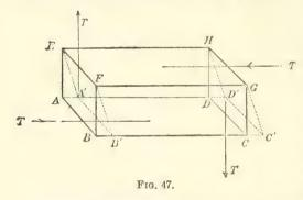
point, so that there would be a swelling of the tube; reversing the couple applied to the tube would, however, reverse the displacement (since we suppose Hooke's Law to hold); hence a couple in one direction would cause the tube to swell, while one in the opposite direction would cause it to contract; it is evident, however, that whether the tube swells or con-
