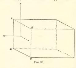
most general force which can act on a face ABCD of the cube may be resolved into three components, one at right angles to ABCD, the other two components in the plane of ABCD, one parallel to AB. the other to BC: similarly over the other faces of the cube we may suppose similar forces to act. These forces are called stresses; the component at right angles to a face is called a normal stress, the component parallel to the face a tangential stress. The intensity of any component of
