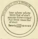
FIG. 10.—Principle of Airy's Harton Pit Experiment.
