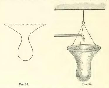
it as in Fig. 94, and gradually fill the vessel with water and watch the changes in the shape of the membrane, these will be found to correspond closely to those in the drop of water falling from the tube; the stage corresponding to that immediately preceding the falling away of the drop is especially interesting; a very marked waist forms in the membrane at this stage, and the water in the bag falls rapidly and looks as if it were
