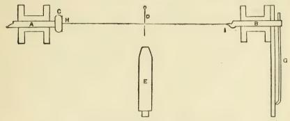
FIG. 7.-Threlfall and Pollock's Quartz-thread Gravity Balance.
