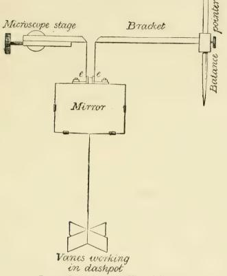
FIG. 15 .- Double Suspension Mircor (half size).
