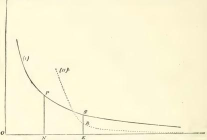
FIG. 24.-Ourve showing the Elastic After-effect in a Twisted Glass Thread.
