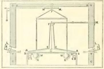
FIG. 11.—Cavendish's Apparatus. h h, torsion rod hung by wire l g; x x, attracted balls hung from its ends; W W, attracting masses movable round axis P. T T, telescopes to view position of torsion rod.
