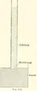
the pot and compress the air in the gauge, the pressure in the pot increasing until a definite pressure is reached depending on the strength of the solution. When this pressure is reached there is equilibrium, and there is no further increase in the volume of water in. the pot.
