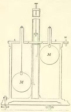
FIG. 12.—Diagrammatic Representation of a Section of in diameter. The torsion Boys's Apparatus. rod N was 0.9 inch long
