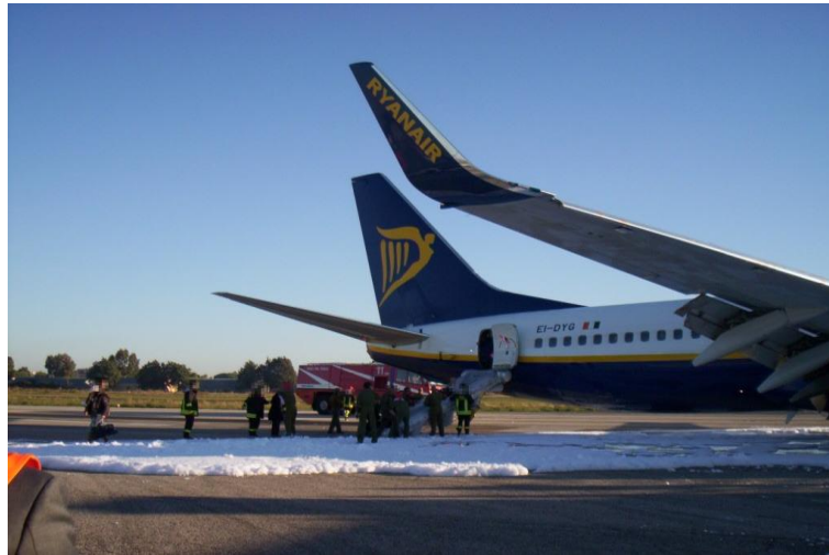
Photo 23: passengers evacuation through the rear right door slide.
