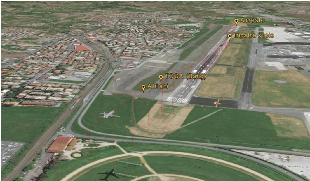
Figure 27: ANSV reconstruction of the final trajectory of EI-DYG.
