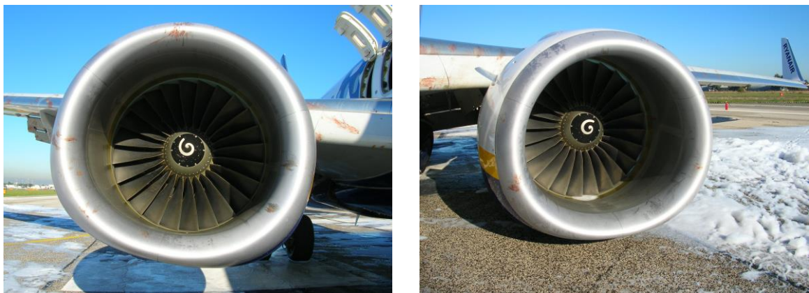
Photos 17 and 18: bird strikes on the engine air intakes.
