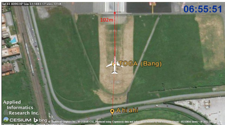
Figure 37: engine stalling point and bird strike.
