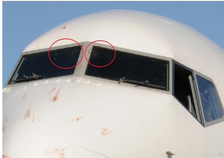
Photo 10: bird strikes on the windshield panels.
