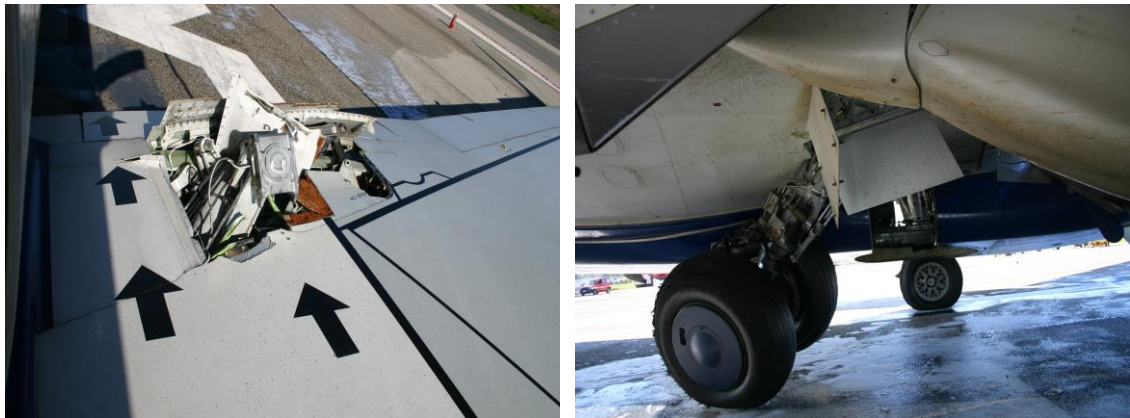
Photos 15 and 16: damage to the main left hand landing gear and wing.
