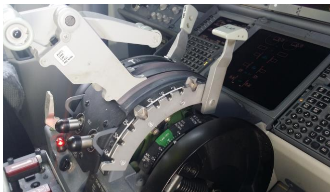
Photo 1: flap command lever.
