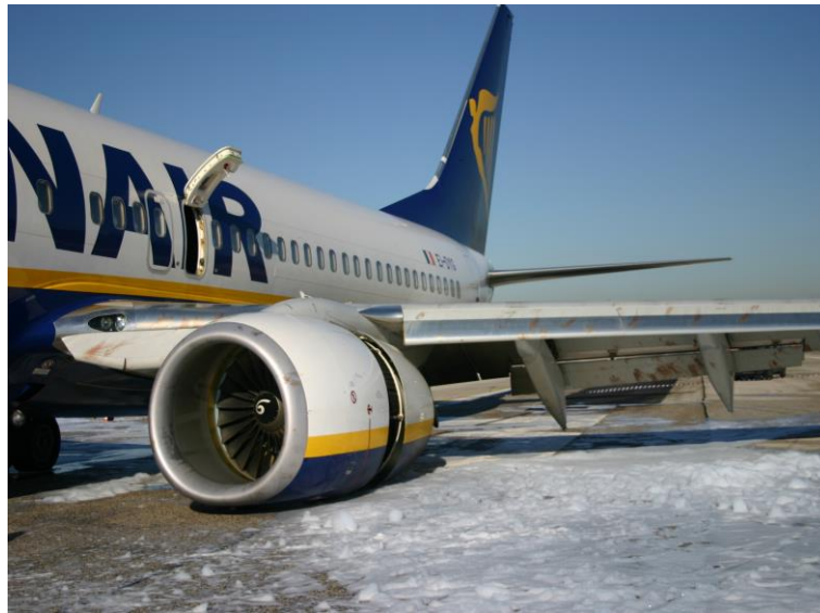
Photo 19: thrust reverse locked in partially open position.
