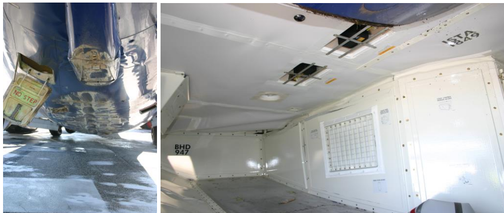
Photos 11 and 12: damage to the tail and passenger floor structure.
