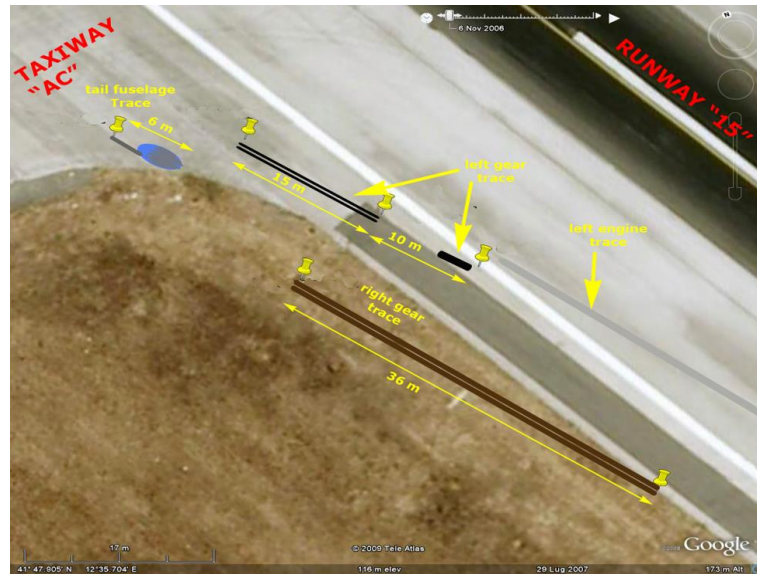
Photo 6: overall view of the landing gear and tail fuselage marks on the ground.
