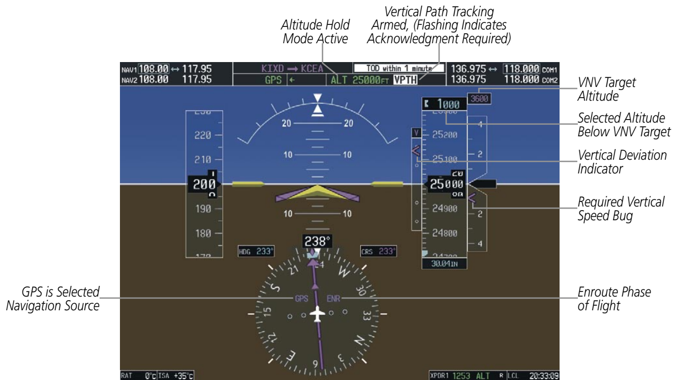
Figure 7-14 Vertical Path Capture
