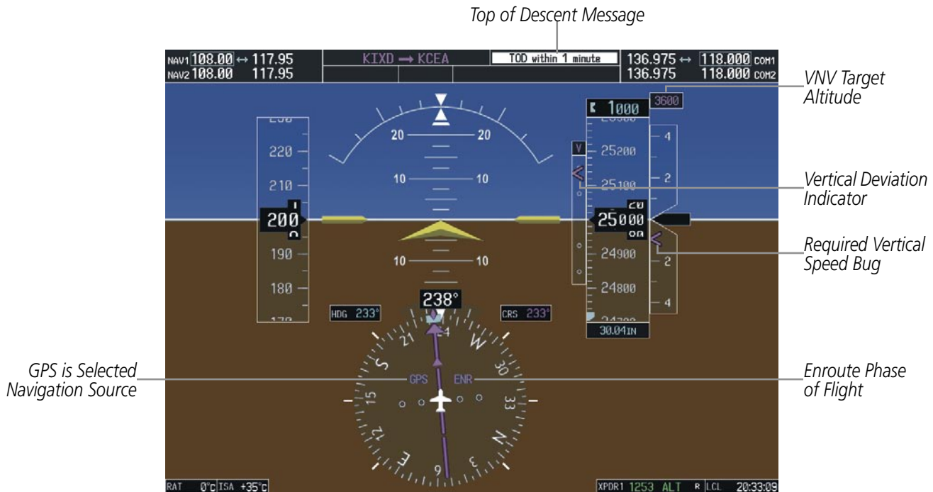
Figure 2-35 Vertical Navigation Indications (PFD)
