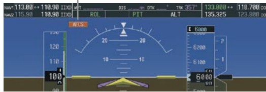
Figure A-5 AFCS System Status Field
