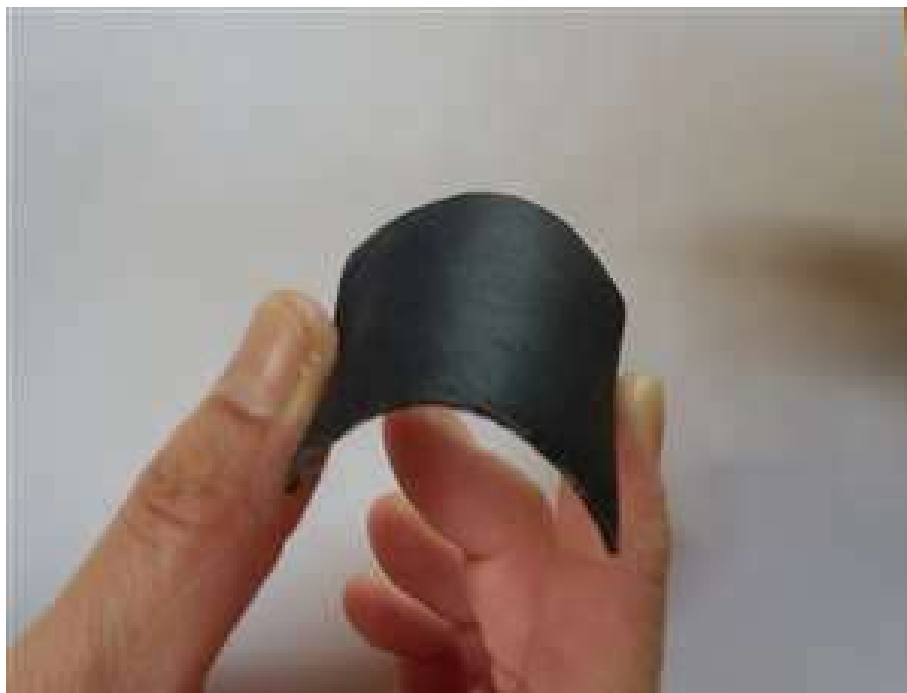
Pic1 薄く軽く曲がる正極集電体
