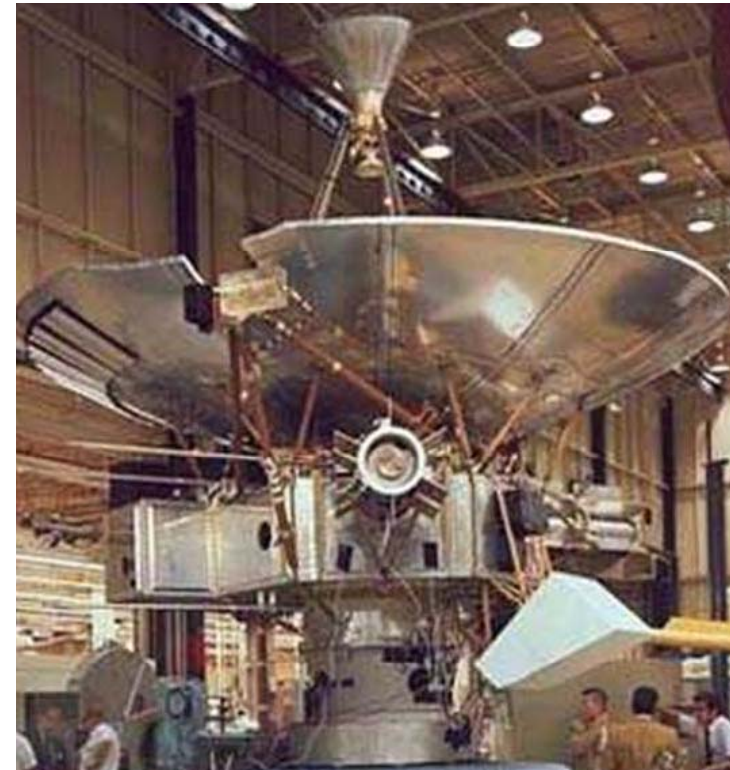
Test Article in Thermal Model Test (Mix of Flight and Non-flight H/W)
