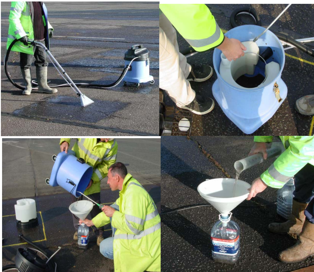
FIGURE 4 Wet washing of the test surfaces and transfer of the salt solution into a container.
