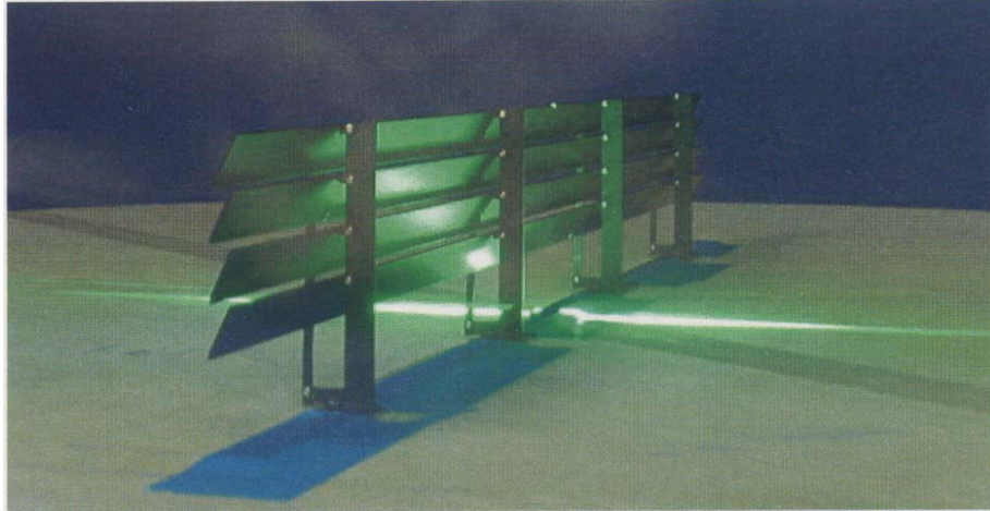
FIGURE 2 Model blower snow fence (11 cm high).
