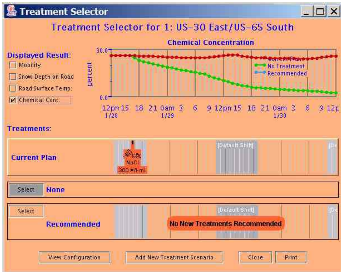
FIGURE 6 MDSS treatment selector screen. The red trace (top line, top window) shows the predicted chemical concentration if the treatment application is followed. The green trace (bottom line) shows the chemical dilution rate if no chemicals were applied.
