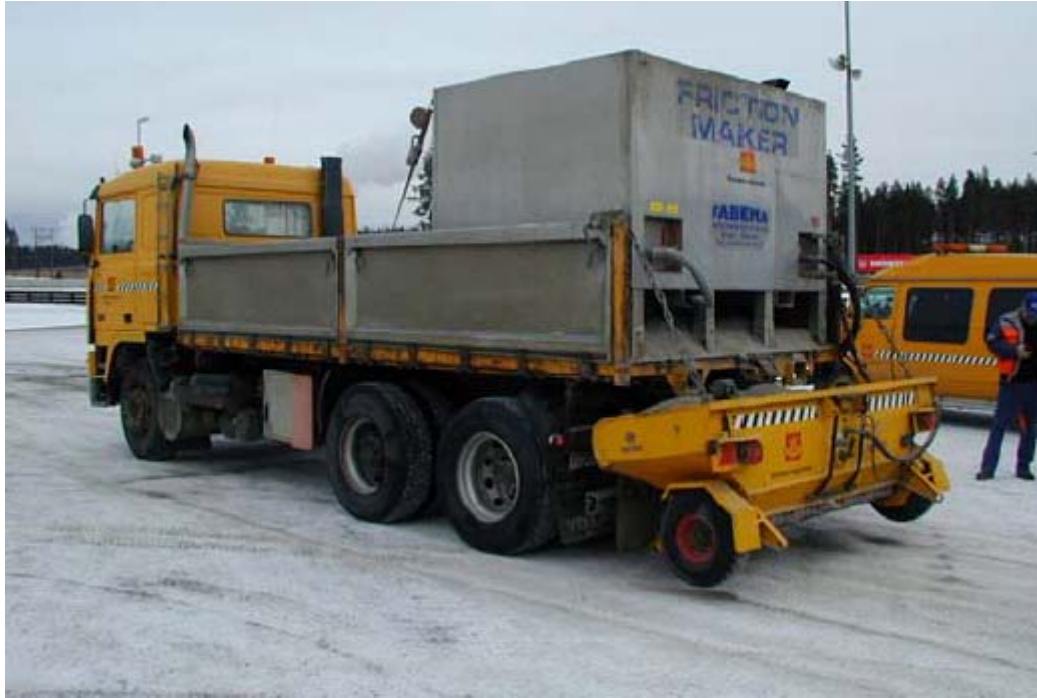
FIGURE 2 Swedish prototype for warm wetted sand.
