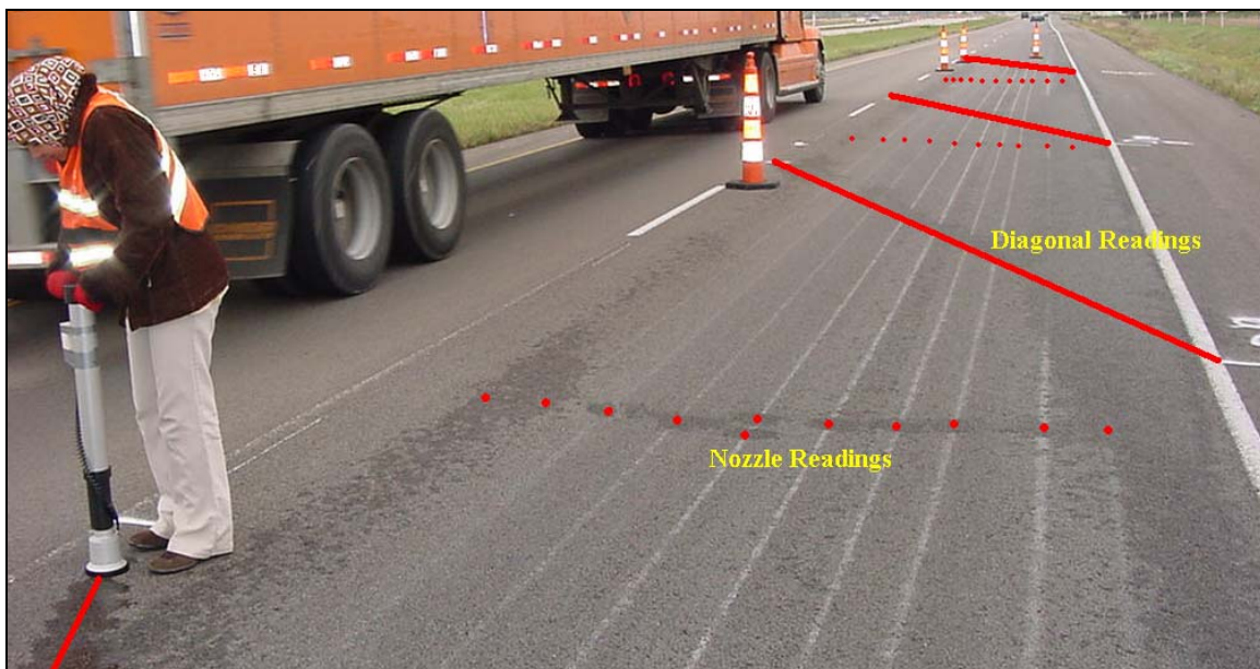
FIGURE 1 Brine residual measurements along the pavement diagonal and on the brine lines.
