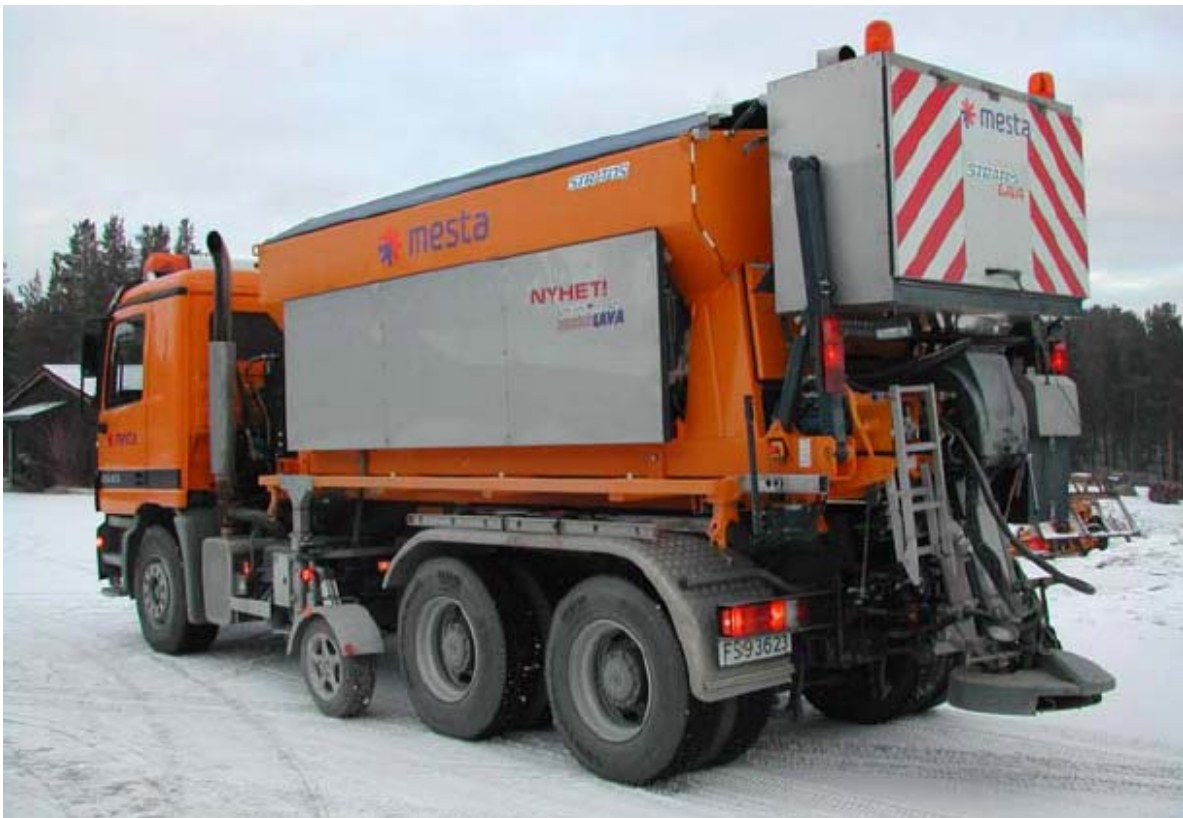
FIGURE 14 Warm wetted sand spreader with friction device.
