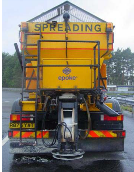
FIGURE 1 A typical prewetter salt vehicle used in the UK.
