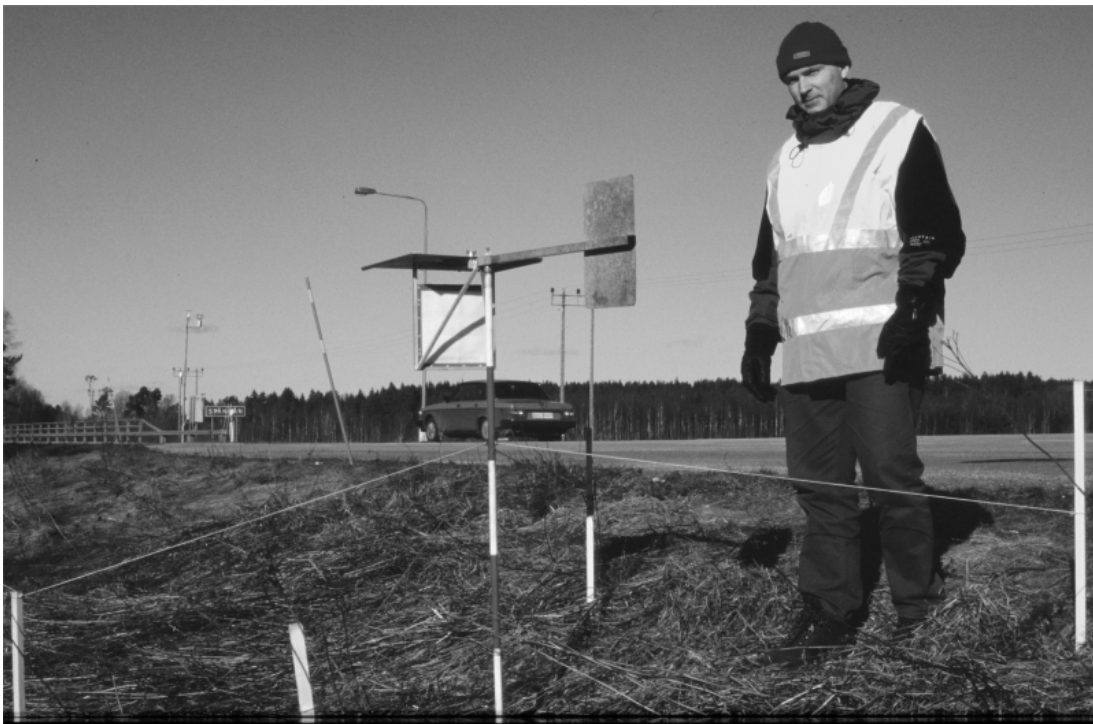
FIGURE 3 Salt vane at the Vimmerby field site.
