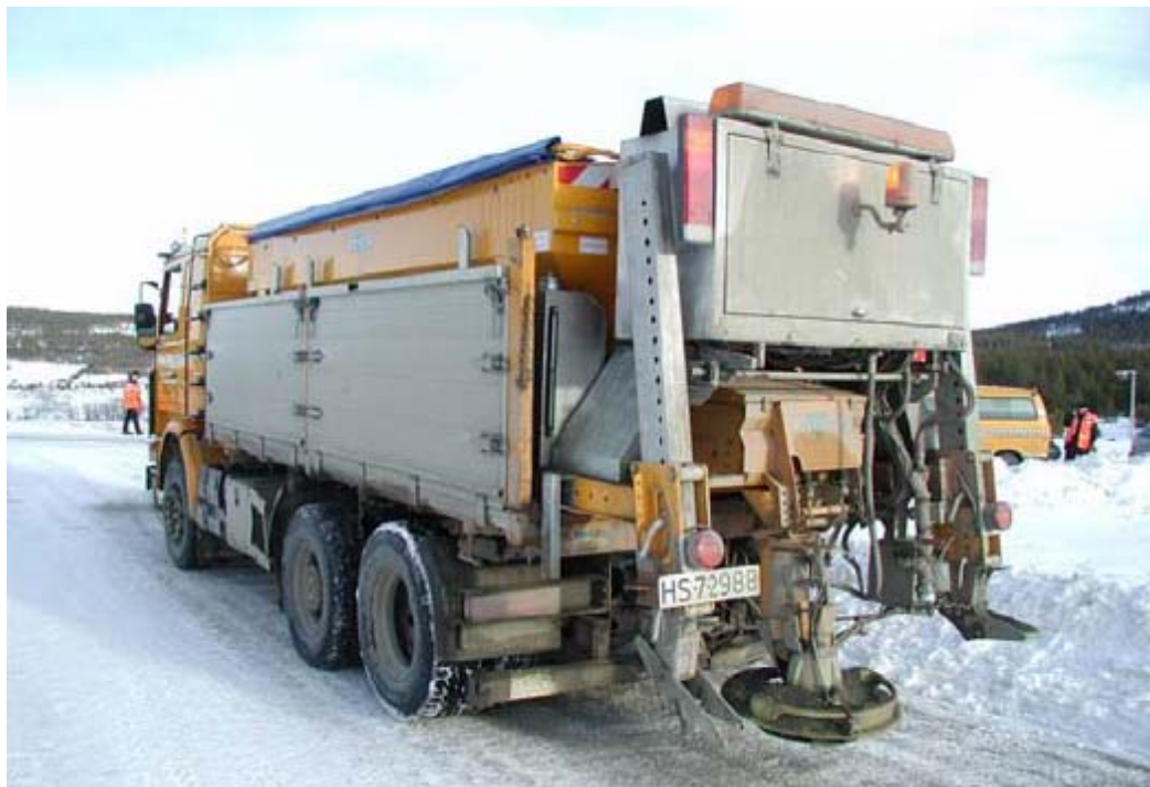
FIGURE 3 New concept for warm wetted sand spreader.
