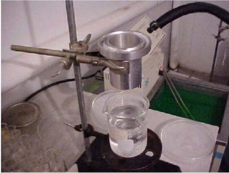
FIGURE 1 Viscosity measured with a Ford #2 cup viscometer.
