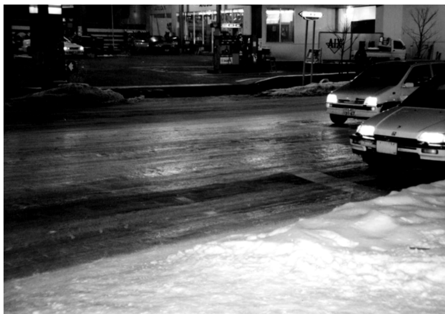
FIGURE 2 Extremely slippery crosswalk caused by studless tires.
