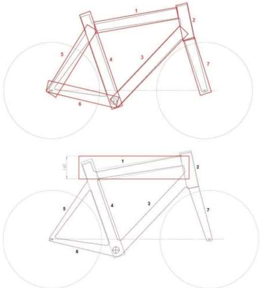
Tubes 1, 2, 3, 4 : 2.5cm minimum & 8cm maximum Tubes 5, 6, 7 : 1cm minimum & 8cm maximum
