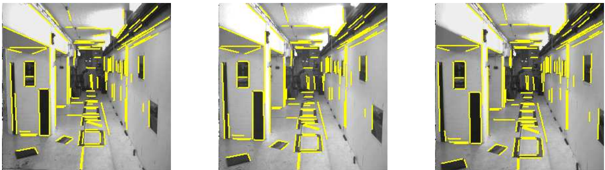
Figure 26: Three view line matching III : The images are 512 \times 512 pixels. There are 282/285/285 line segments in the first/second/third views. Of these 130 are matched, all the line matches are correct.
