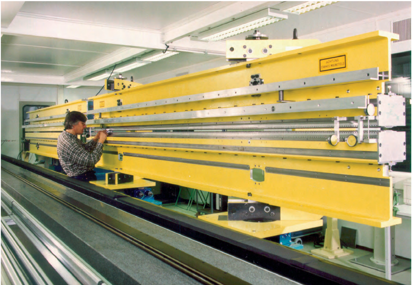
Photo of a FLASH undulator magnet. The gap height is 12 mm, the period is \lambda_u = 27 mm and the peak magnetic field is B_0 = 0.47 T.
