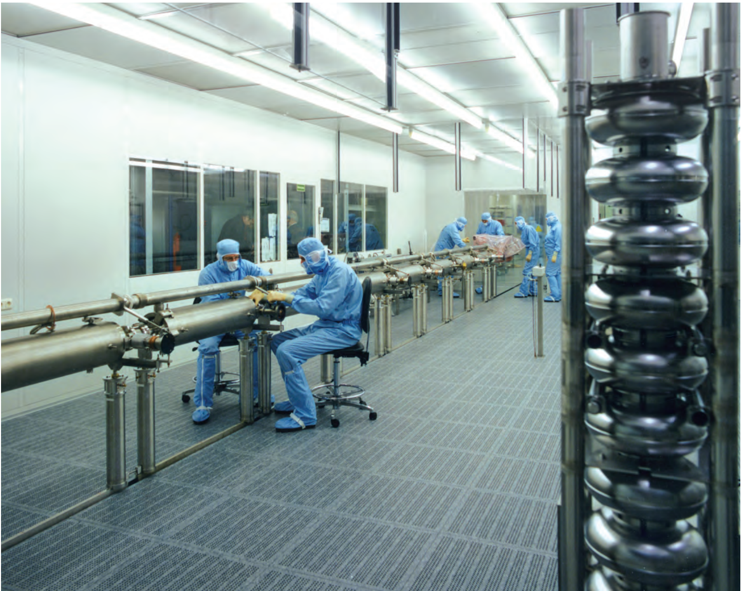
Preparation of the superconducting cavities in the DESY cleanroom: A string of eight cavities, each welded into its own liquid-helium tank, is being assembled and prepared for installation in an acceleration module. On the right: a single nine-cell cavity equipped with vacuum flanges and a radio-frequency input coupler for the performance test in a liquid-helium bath cryostat.
