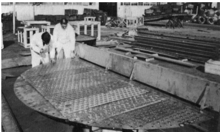
A typical stainless steel valve cap tray that might be used in a fluid catalytic cracker gas treating plant.
