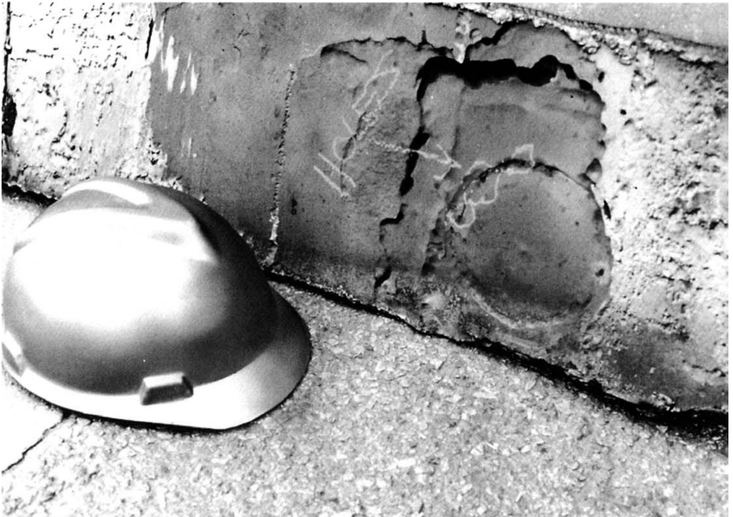
Figure 43 Absence of scale and grooving of the metal surface are characteristic of naphthenic acid corrosion of carbon steel. Type 316 stainless steel has excellent resistance to attack by naphthenic acid.
