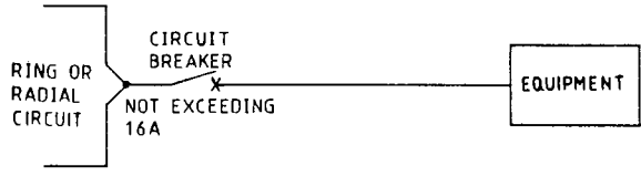
(B) CIRCUIT BREAKER PROTECTION
