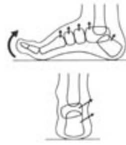
図2 Windlass type Mechanism
