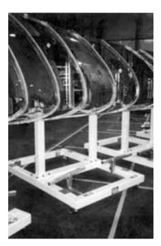
When investigators pieced together the debris from the wreckage of the space shuttle Columbia, they loaded the gray reinforced carbon-carbon (RCC) heat shields from the leading edge of the left wing in a plastic frame and determined that falling foam had punched a hole in shield number 8 (shown above). This allowed superhot gases to flow past the breach during reentry, leading to the disaster. From Final Countdown.
