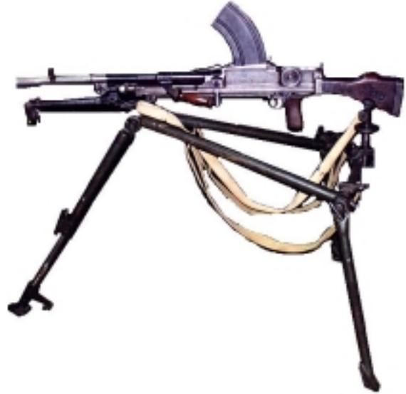
TOP: A British Bren MG mounted on a tripod mount for use in a sustained fire role. Courtesy of Gary Crocker, photo by Michael Dorosh.
