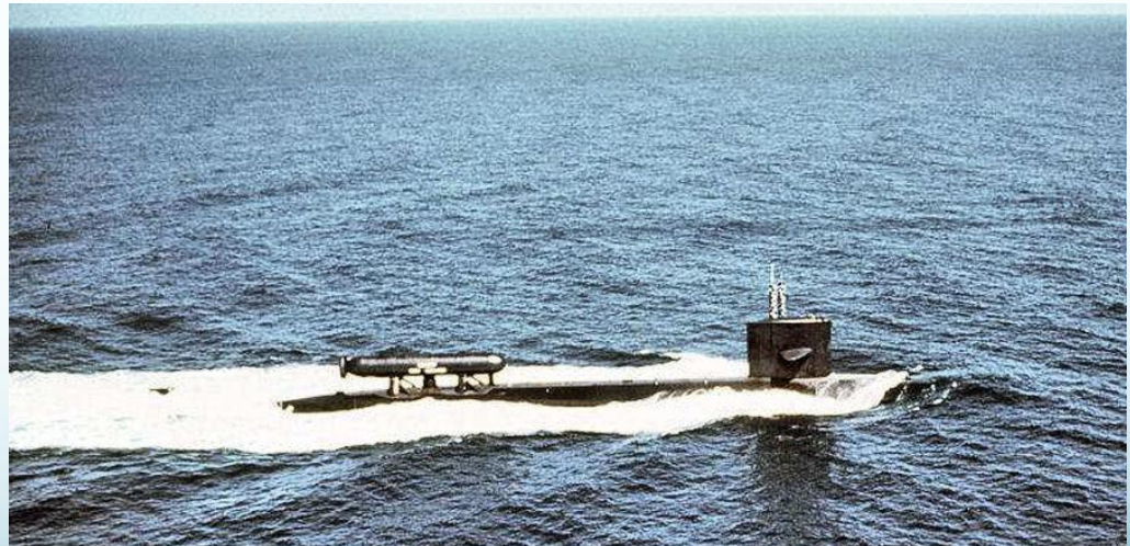
Parche circa 1983. The “DSRV-look-alike” structure on the boat’s aft section was a lock in-lockout chamber for saturation divers Source: www.navsourc.org
