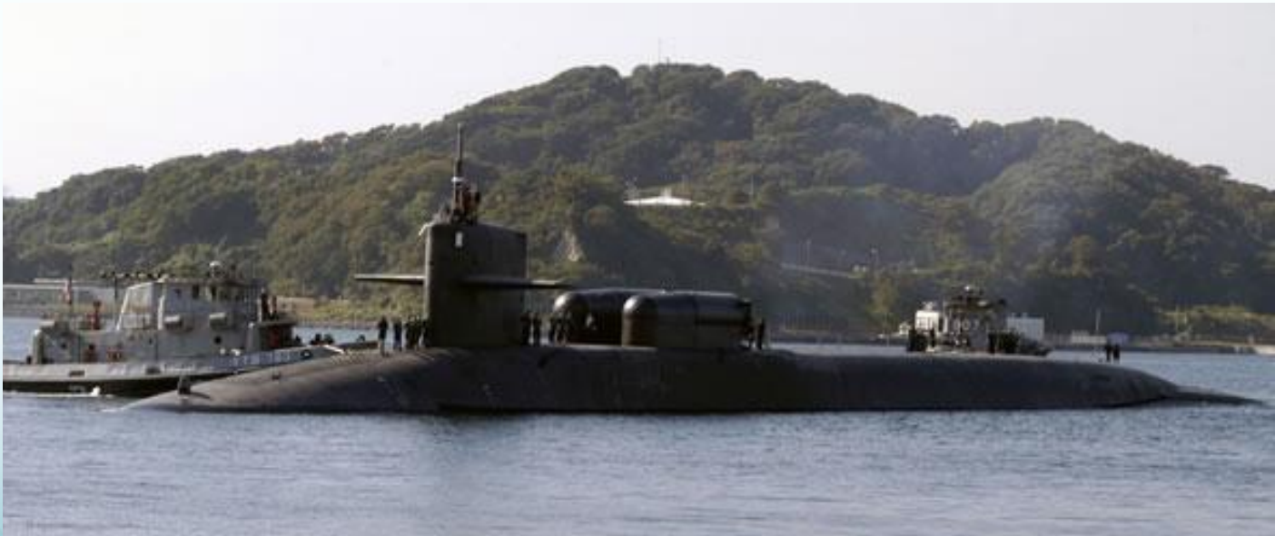
Ohio with 2 x Dry Deck Shelters for Special Operations Forces (SOF)
