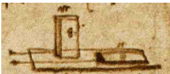
Fig. 5 Sketch showing a block of weight 8 units sliding in two different orientations labelled m and n (CA 198r, c. 1508)
