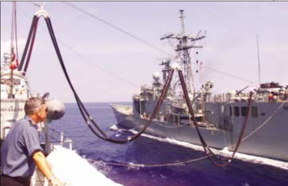
Versatile and Capable: HMCS Protecteur refuelling a RAN frigate — East Timor — 1999 (CF Photo)
